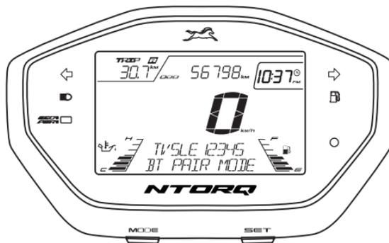
5. The connected instrument cluster's Bluetooth name is prefixed by TVSLE and followed by alpha-numeric digits. Ex : 'TVSLE12345'. This Blue-tooth name can be found by changing the cluster mode into BT pair mode.
