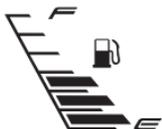
When the fuel reaches minimum safe level (1.5 liters approx.), the last bar of the fuel gauge starts blinking and low fuel indicator starts glowing. The message 'FUEL ON RESERVE' will be displayed at alpha numeric display and 'TRIP F' meter starts counting from 0.0 km as explained in page No. 19.
