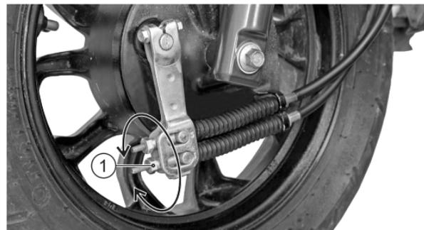
5. If any clearance is found, turn the adjuster nut (2) at the top side in the slot marked as "S" in clockwise direction until there is no clearance between the bullet top (3) and the slot top (4).
