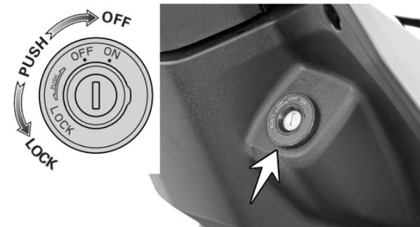
The engine can be started. Control key cannot be taken out from the lock.
