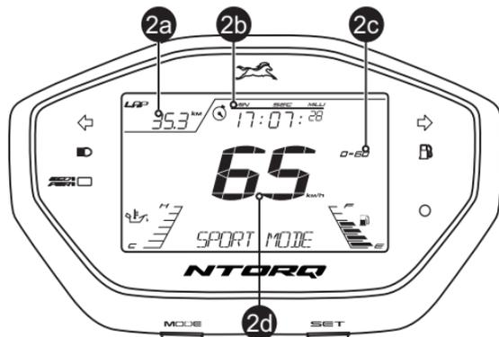
To enter into sport mode, short press the 'Mode' button in street mode while 'Trip B' in display.
